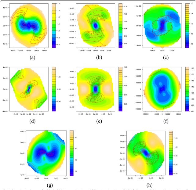
**Fig. 3** Smoothed variogram of residuals of *PGV* at record stations of different earthquakes; **a** Chi-Chi, **b** Chuetsu, **c** El Mayor, **d** Iwate, **e** Niigata, **f** Northridge, **g** Parkfield, **h** Tottori
