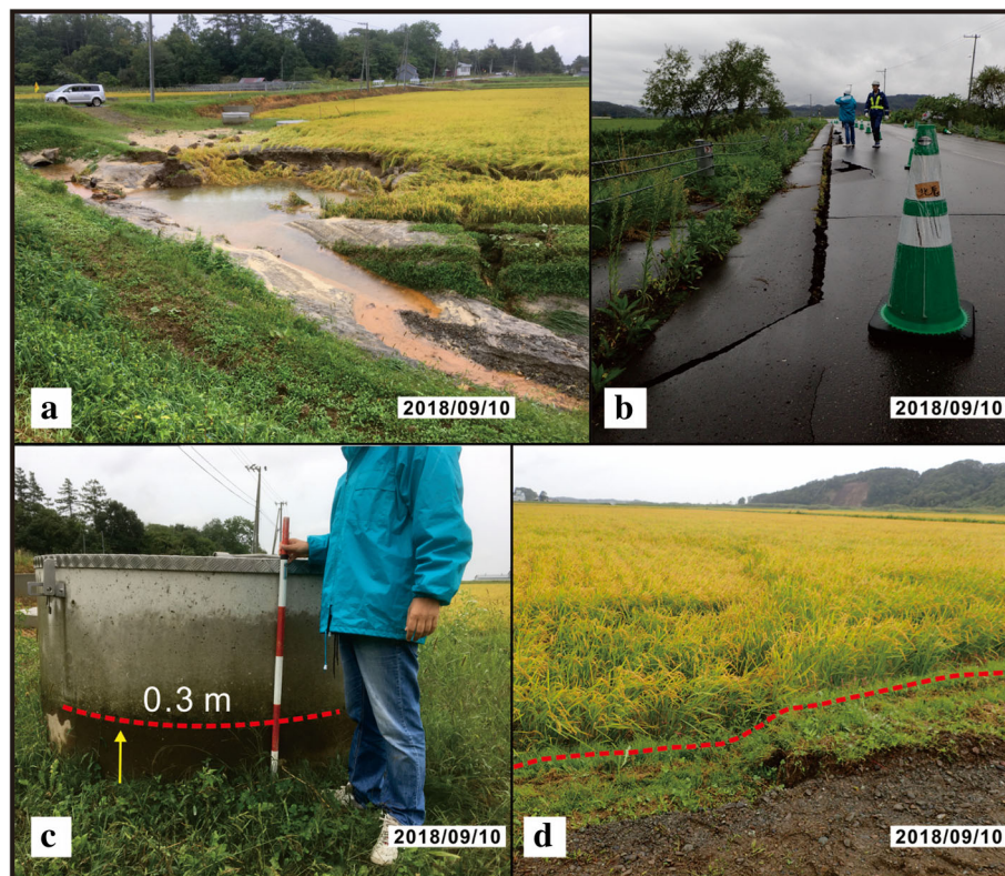
Fig. 3 Damages and liquefactions resulted from the Iburi earthquake sequence. a Liquefaction and jetted sand in the paddy field. b Road damage. c Uplift of inlet well. d Surface rupture in the paddy field
