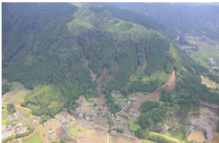
Fig. 1 Shallow landslides on the northeastern rim of Aso caldera (image courtesy of Kokusai Kogyo Co., Ltd, Japan)
