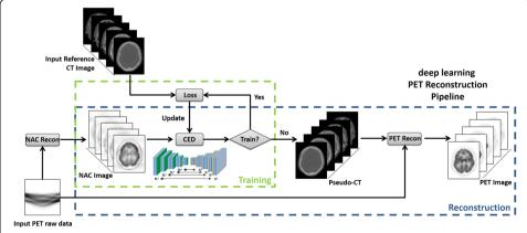
**Fig. 2** Schematic illustration of deepAC. The process consists of a training phase and a reconstruction phase. The training phase is first performed with NAC and co-registered CT data, after which the well-trained network is fixed and ready for generating pseudo-CTs for new PET data in the reconstruction phase
