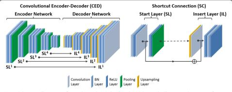
**Fig. 1** Schematic illustration of convolutional encoder-decoder in this study. This network consists of multiple symmetrical shortcut connection (SC) from the start layer (SL) in the encoder to the insert layer (IL) in the decoder. The insertion of SC follows the strategy of the deep residual network described in Reference [22]
