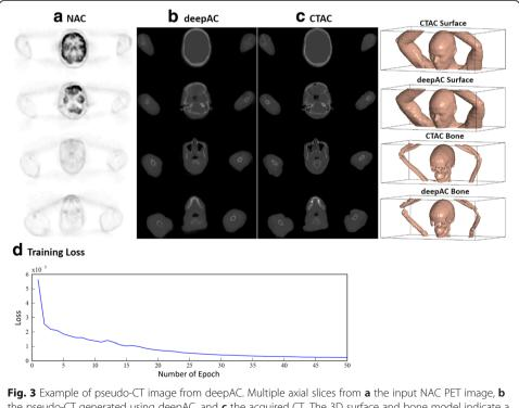
**Fig. 3** Example of pseudo-CT image from deepAC. Multiple axial slices from **a** the input NAC PET image, **b** the pseudo-CT generated using deepAC, and **c** the acquired CT. The 3D surface and bone model indicate a high similarity between the acquired CT and pseudo-CT. The surface and bone were rendered using a HU value of -400 and 300, respectively. The training loss curve is shown in **d**
