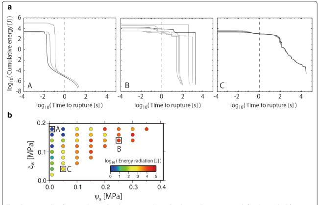
**Fig. 7** Parameter studies of energy radiation. **a** Cumulative energy radiation plotted against the time remaining before the mainshock for parameter sets A–C. Black curves represent events presented in Fig. 3. Grey curves are for other mainshocks shown in Fig. 2. **b** Results of parameter studies. The color indicates the amount of cumulative energy at 1 s before the mainshock. Parameter sets A–C shown in **a** are denoted by squares
