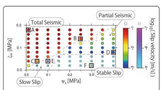
**Fig. 4** Phase diagram for different types of slip behavior. Color intensity represents slip velocity. Symbols (circles and squares) denote the color scale used. The six parameter sets shown as examples in Figs. 2 and 3 are indicated by text labels **A–F**
