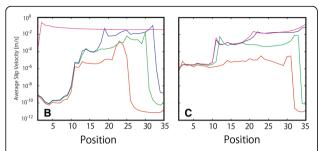
**Fig. 9** Snapshots of slip velocities on the fault for parameter sets **B** and **C**. Green line shows the slip velocity at the beginning of the mainshock, when the average slip velocity exceeds 1 mm/s, corresponding to the insets in Fig. 5a. The blue and magenta lines are snapshots when the averaged slip exceeds 1 cm/s and reaches its maximum, respectively. The red line is a snapshot taken 1 s before the beginning of the mainshock
