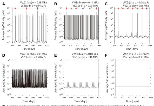
**Fig. 2** Examples of simulation results. The slip velocity averaged in the seismogenic zone is shown for parameter sets **A–F**. Arrows in **A–C** represent the times of mainshocks. Detailed slip behavior of mainshocks denoted by blue arrows is shown in Fig. 3
