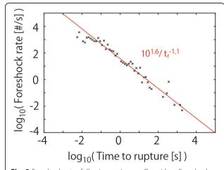
**Fig. 8** Foreshock rates following an inverse Omori law. Foreshock rates measured for the stacked sequence in parameter set B are shown against the time remaining before the mainshock. The red line denotes the fitted power law function. Estimated parameters are shown in the plot with red text
