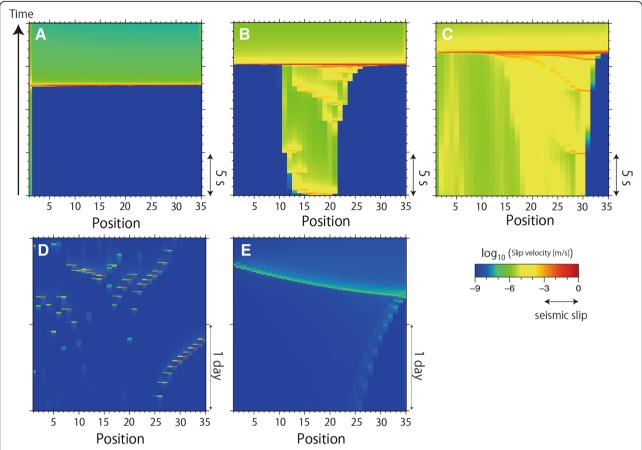
Fig. 3 Detailed slip behaviors of the fault. Five examples (parameter sets A–E in Fig. 2) are shown, one per panel. Horizontal axis shows the location (referenced by cell number) along the fault (cf. Fig. 1). Time flows from bottom to top on the vertical axis. Color intensity corresponds to slip velocity in each cell as a function of time
