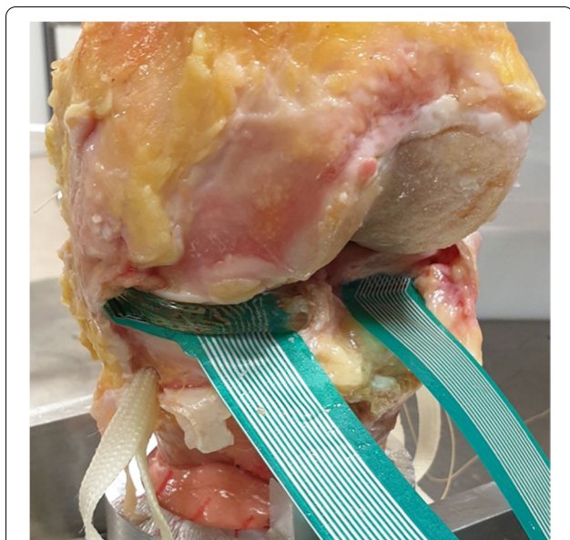
Fig. 9 Second-generation meniscus prosthesis and sensor in a cadaveric knee joint
