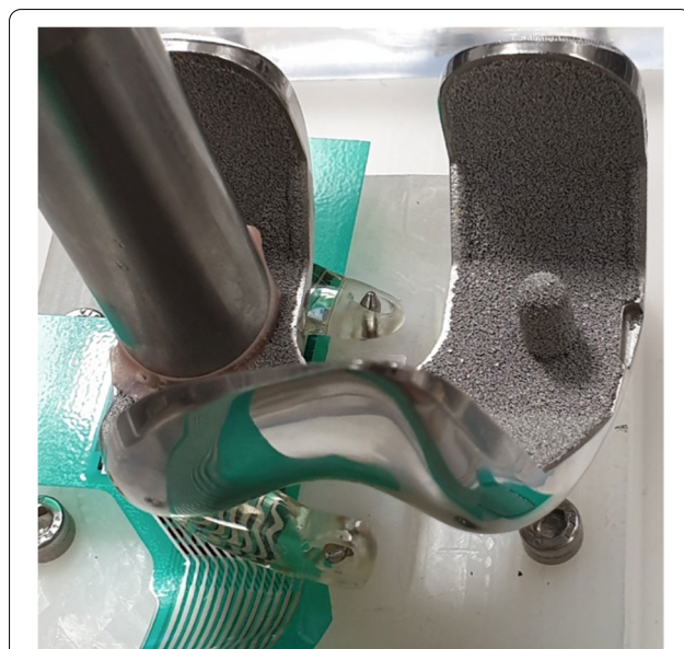
Fig. 7 First-generation meniscus prosthesis and sensor in the artificial knee joint
