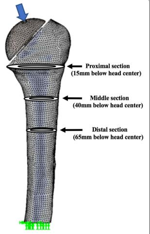
**Fig. 3** Meshed model of an implanted humerus, rigidly fixed at the distal part, indicating the direction of the proximal load towards the center of the prosthetic head
