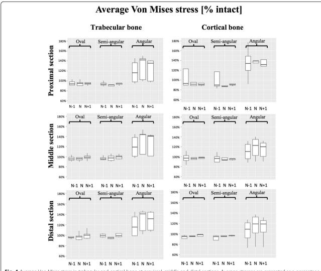
Fig. 4 Average Von Mises stress in trabecular and cortical bone at proximal, middle and distal sections. Average stresses are presented as a percentage of the intact bone stress in each section
