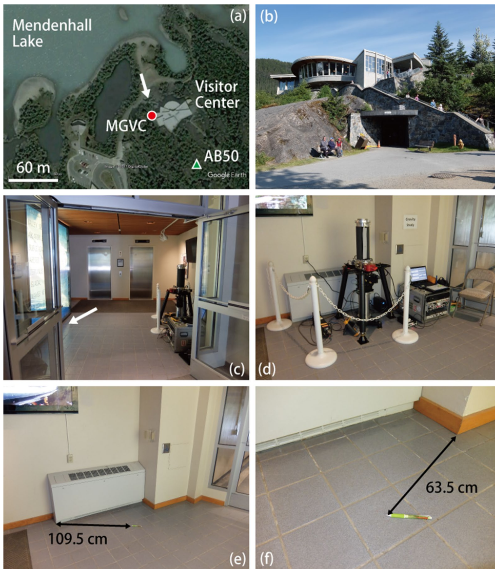
Fig. 14 Location of the MGVC gravity point. a The satellite image of Mendenhall Glacier Visitor Center derived from Google Earth Pro. The red circle and green triangle indicate the MGVC gravity point and AB50 GNSS station, respectively. The white arrow indicates the direction of the photo (b) . b The entrance of Mendenhall Glacier Visitor Center. MGVC is located about 25 m from the entrance. c The elevator lobby of the Mendenhall Glacier Visitor Center, where the AG point is located. The new AG point is located on the right side of the lobby when facing the elevators. The old AG point (Sun et al. 2010) was located at the left side of the lobby. However, in June 2012, we found that the old point was not available because of the illuminating exhibition. The white arrow indicates the photo direction of Figure A5 in Sun et al. (2010). d The FG5-111 absolute gravimeter on the new AG point. e The position of the new AG point. It is located at the tip of the pen and approximately 109.5 cm from the corner of the heater. The heater should not be activated during the AG measurement, because its vibration magnifies the scatter of the AG data. f The exact position of the new AG point. It is located at the center of a tile and approximately 63.5 cm from the corner of the pillar. Note that we failed to measure the gravity difference between two AG points using a relative gravimeter directly during the campaign AG measurement in 2012, due to the exhibit installed on the old point by the visitor center. Instead, we considered the gravity difference by adding a term of the step-like gravity change between 2008 and 2012 in reproducing the temporal gravity change at MGVC (Fig. 5)
