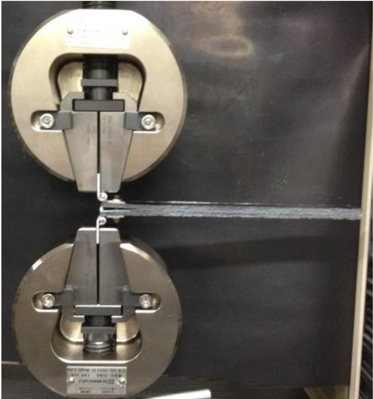
Figure 3 Mode I test of DCB specimen consisting of GFRTF.
