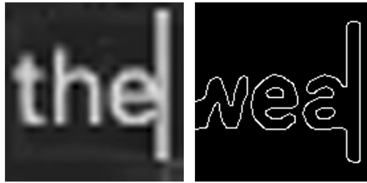
Fig. 5 Sticking characters problem, where a character seems visibly merged with text cursor due to low-resolution frame
