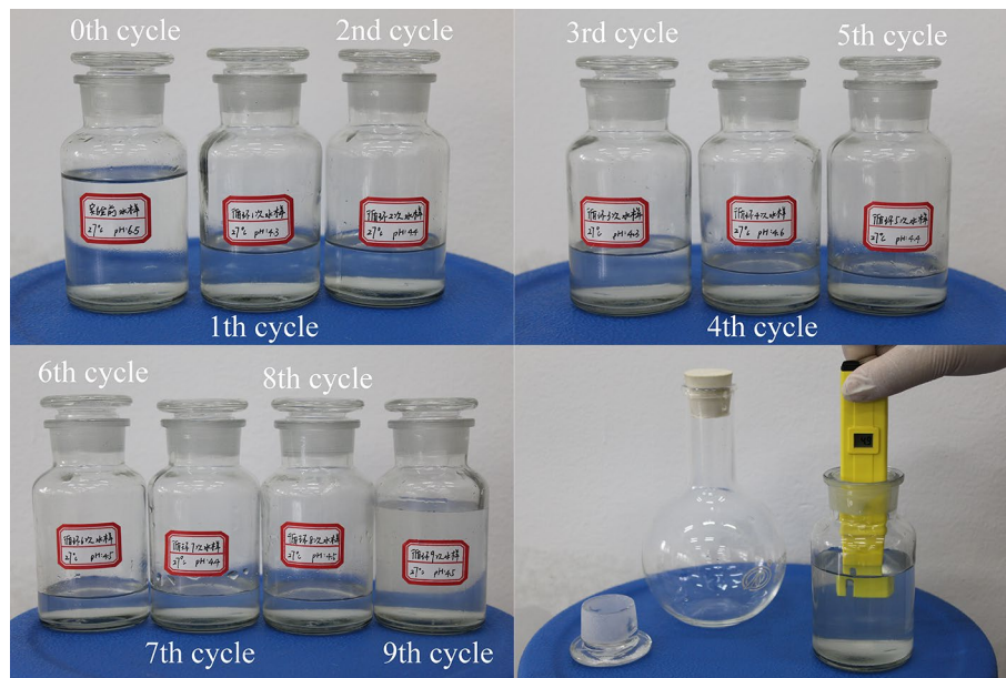
Fig. 3 Fracture water samples collected during each injection cycle for rock sample CA-2 and pH testing
