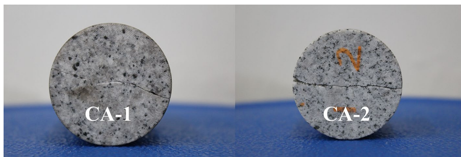
Fig. 2 Fractured granite samples CA-1 and CA-2 without proppant
