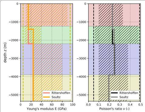
**Fig. 6** Comparison of Young's modulus (left) and Poisson's ratio (right) between Rittershoffen and Soultz-sous-Forêts sites. The shadow zones correspond to the range of experimental values (Young's modulus in yellow, and Poisson's ratio in gray) (see Table 1). The dashed lines correspond to boundaries of the prior distributions for the back analysis (see Table 3). Background colors correspond to geological units
