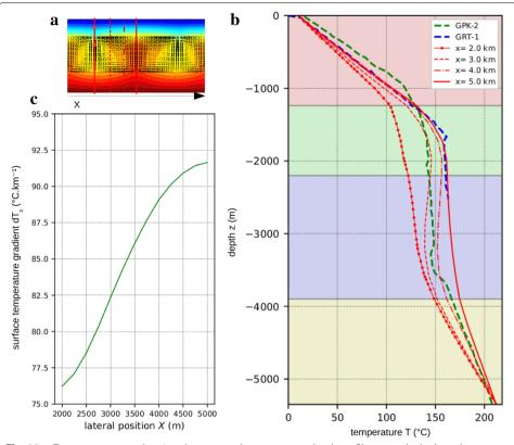
**Fig. 11 a** Temperature map showing the extracted temperature–depth profiles to study the lateral temperature variability. **b** Simulated vertical temperature profiles (as red lines) obtained every kilometer along a half-convection cell compared with the observed GRT-1 log from Rittershoffen (as blue dashed line) and GPK-2 log from Soultz-sous-Forêts (as green dashed line). **c** Thermal gradient obtained from the surface obtained every kilometer along a half-convection cell
