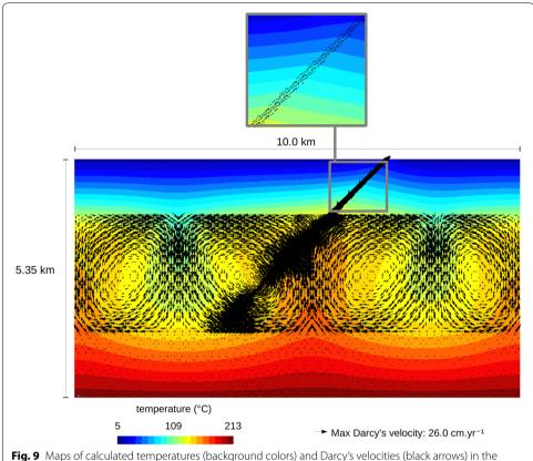
**Fig. 9** Maps of calculated temperatures (background colors) and Darcy's velocities (black arrows) in the model including the Rittershoffen fault with dip of 45°
