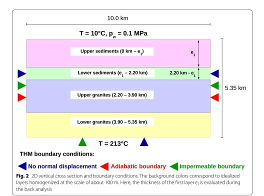
This idealized cross section is 5.35 km in height and 10 km in width and contains no large-scale fault. Below, we denote by x the horizontal direction, z the out-of-plane horizontal direction and y the vertical one. The typical size of elements is 100 m  $\times$  100 m. Consequently, the rheological properties taken as inputs as the model are homogenized at this length scale. In Fig. 2, the boundary conditions used in our numerical simulations are also summarized:
