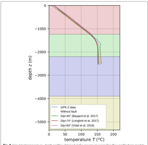
**Fig. 7** Simulated temperature—depth profiles obtained at the maximum ascending flow profile from models including the Rittershoffen fault with different dips and compared to the model without fault
