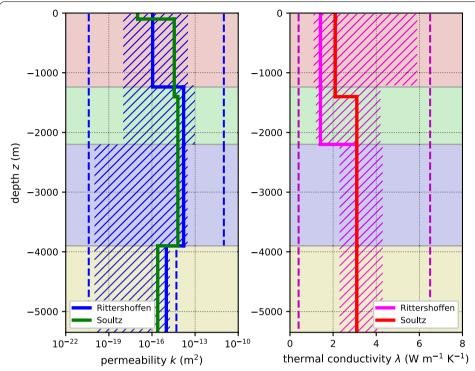
**Fig. 4** Comparison of permeability estimated by back analysis (left) and thermal conductivity (right) between Rittershoffen and Soultz-sous-Forêts sites. The shadow zones correspond to the range of experimental values (permeabilities in green, and thermal conductivity in red) (see Table 1). The dashed lines correspond to the prior distributions for the back analysis (see Table 3). Background colors correspond to geological layers
