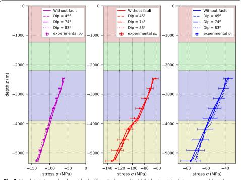
**Fig. 8** Simulated stress-depth profiles [(left) vertical  $\sigma_v$  and (middle) horizontal minimum  $\sigma_h$  and (right) maximum  $\sigma_{H}$ ] obtained at the maximum ascending flow profile from models including the Rittershoffen fault with different dips and compared to the model without fault
