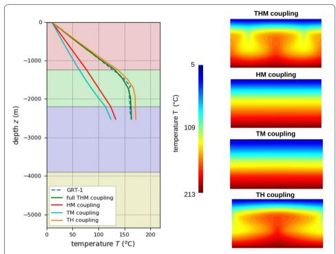
**Fig. 10** Left: comparison of temperature–depth profiles for four studied cases: in green, the full coupling between thermic, hydraulic and mechanic processes is taken into account; in red, the coupling is only between hydraulics and mechanics; in blue, between thermics and mechanics; and in orange, between thermics and hydraulics. Right: associated maps of temperatures
