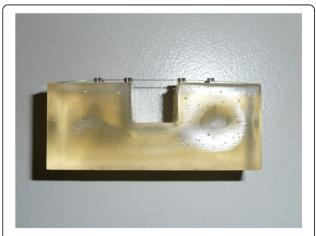
Fig. 3 Mounted archwire on the acrylic resin base
