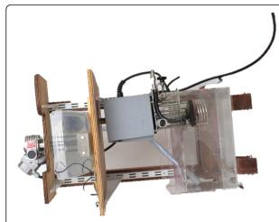
**Fig. 2** Aging machine composed by the gear motor, the stainless steel support, water and saliva baths, and the heating pump
