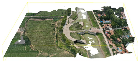
Fig. 5 3D point cloud model of Daiwan Lock (Figure created by the research team)
