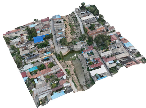
Fig. 9 3D point cloud model of Liangxiang Lock (Figure created by the research team)
