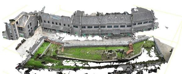
Fig. 6 3D point cloud model of Jingkou lock (Figure created by the research team)
