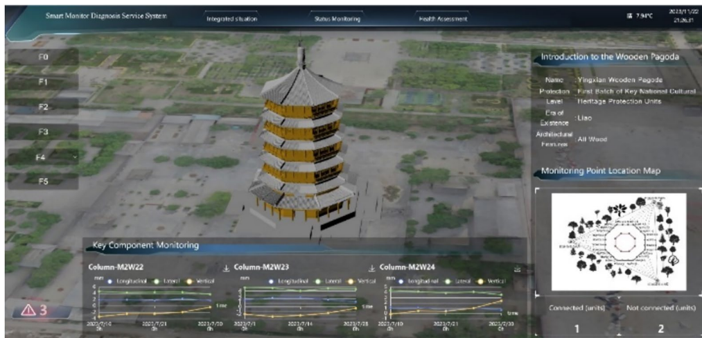
Fig. 16 System presentation diagram for digital twins of ancient buildings
