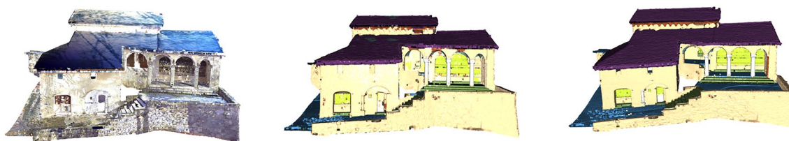
Fig. 10 Front view of 6_SMV_chapel_2to4 (left: original point cloud, center: predicted result, right: real point cloud)
