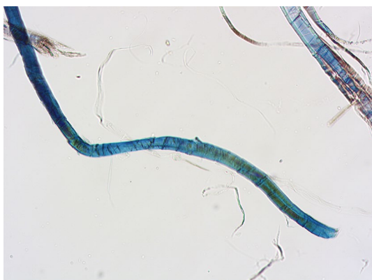
Fig. 19 Blue bast fibre, sample 102, 20×, RV-3025–18
