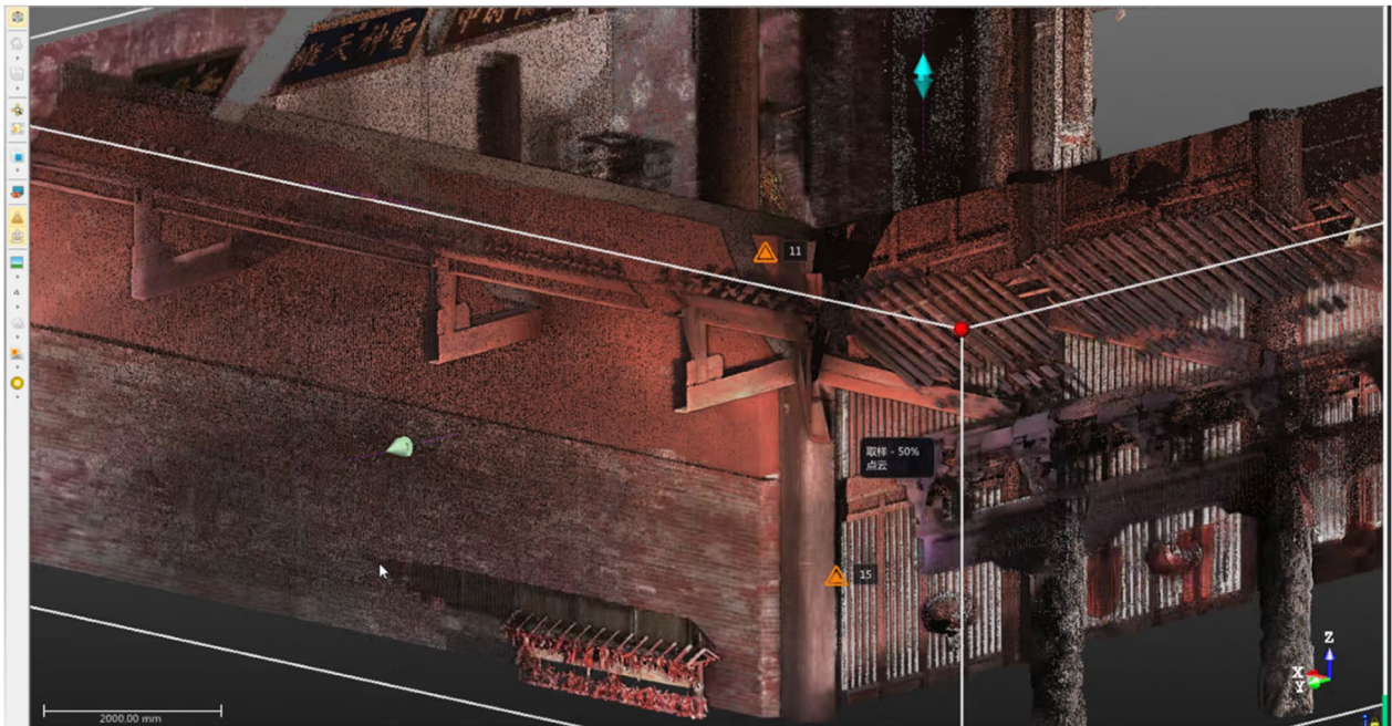
Fig. 16 Point cloud model of the decoration of the pillar head of the Great Achievement Palace
