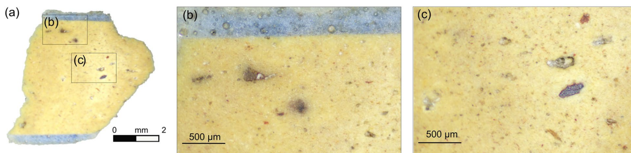
Fig. 4 a Reflection optical microscope image of the polished ceramic fragment displays the glaze surfaces in green-ocean and blue-sky colours. Insets b and c provide detailed views of the external glaze ( b ) and groundmass containing frits, inclusions and amoeboid vesicles ( c )
