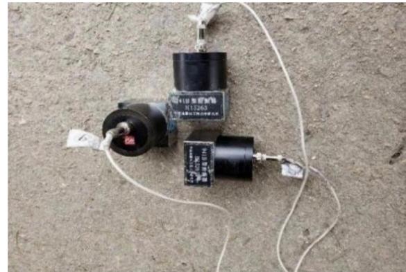
Fig. 3 Position of the vibration picker at the test point
