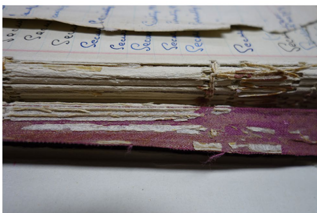
Fig. 3 Detail from FCO 141/13503 showing detached spine with loose and crumbling adhesive (left), and FTIR spectrum of adhesive with reference spectra for gelatine and starch. It is more likely that the carbohydrate signals corresponding to 'starch' in the sample are due to the presence of paper pulp in the glue sample, than starch adhesive
