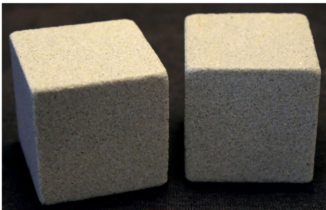
Fig. 1 Photographs of sandstone cubes with size of 50 \times 50 \times 50 \text{ mm}^3 serving as the primary specimens
