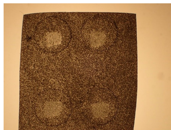
Fig. 6 Transmitted-light photograph of a parchment sample which underwent a short bath [5 min] in 3% \text{H}_2\text{O}_2 solution. Accumulated charge: 2, 3 (upper left and right spots), 4 and 5 (lower left and right spots) \mu\text{C}/\text{cm}^2 , current 1 nA). The photo was taken after drying
