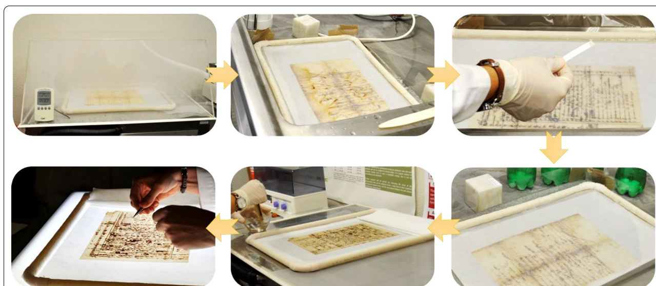
Fig. 4 Calcium phytate main treatment steps: (1) humidification, gradual transition from a dry to a wet state to minimize dimensional tensions in the object; (2) washing in water, for removal of acids and soluble transition metal ions such as \text{Fe}^{2+} or \text{Cu}^{+} ; (3) immersion in calcium phytate solution, complexation of \text{Fe}^{2+} and \text{Fe}^{3+} by phytate; (4) deacidification with calcium bicarbonate, neutralization of remaining acids and deposition of an alkaline reserve in the paper; (5) sizing with gelatine, increasing the mechanical strength of paper and adding a protective layer between the atmosphere and the surface of the ink; and (6) local mending to support areas with mechanical damages and prevent further losses
