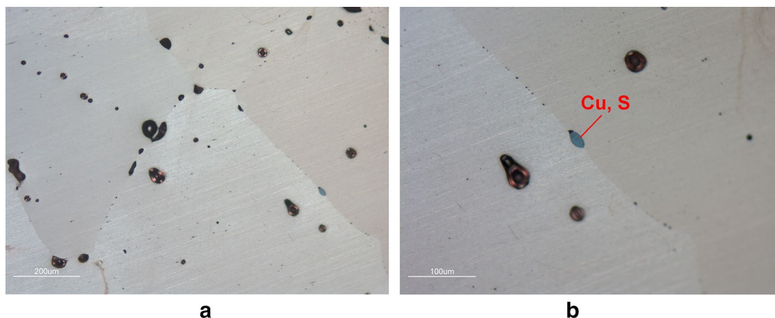
Fig. 11 Cannon from the Old Castle in Grodno, Sample 1—results of metallographic examinations. a, b microstructure in Zone 4, numerous pores and an isolated CuS inclusion (light blue) in the Cu–Pb matrix
