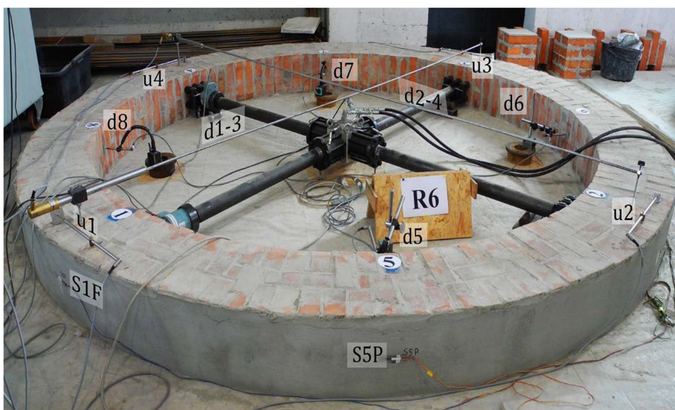
Fig. 4 Model R6 prepared for experimental testing
