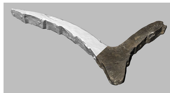
Fig. 8 3D scan of a ship timber, captured with the Artec Eva. Composite image showing the 3D model's base geometry (left) and geometry with texture (right)
