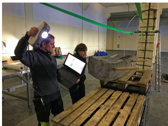
Fig. 7 Scanning a long, flexible plank using the Artec Eva handheld scanner. To avoid changes in shape when the plank is turned over, the plank is suspended above the documentation table and recorded in a single scan
