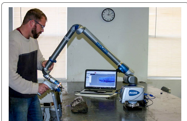
Fig. 5 3D scanning a ship timber, in this case using a laser line probe attached to a FaroArm. Picture reproduced with permission of Christopher Dostal [10]
