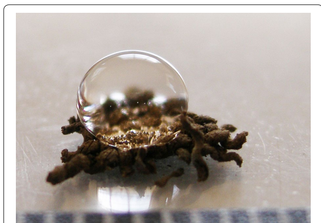
Fig. 1 Unmanipulated image showing how the hydrophobic textile fragment repels a water droplet, which forms a perfect sphere on its surface
