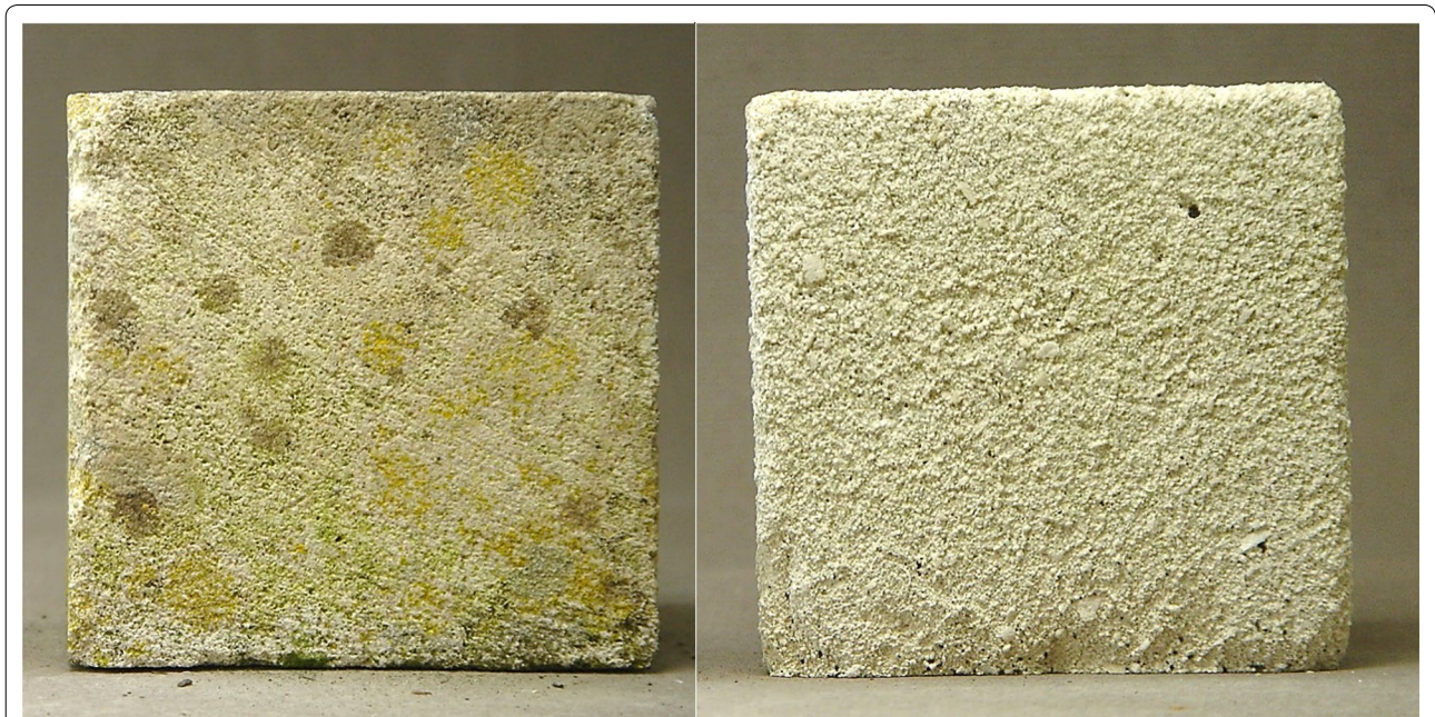
Fig. 6 Visible difference in surface roughness between Portland cubes from Brú na Bóinne 2 (left) and Skellig Michael 3 (right). Photo taken in 2016
