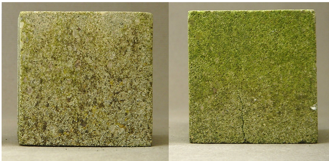
Fig. 2 Micro-climatic effects on biofilm growth: Rock of Cashel Peakmoor cubes 2016, plate one (left) and plate two (right)
