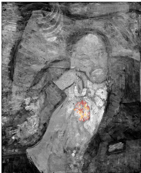
Fig. 16 IRR image (1500–700 nm) with estimated colorization in the region of interest. Using Photoshop CS5, areas of interest in the Hg and Cr SR-XRF maps were selected and converted to red and yellow , respectively. The registered colored layers were superimposed on the IRR image to visualize color in the area of the flower
