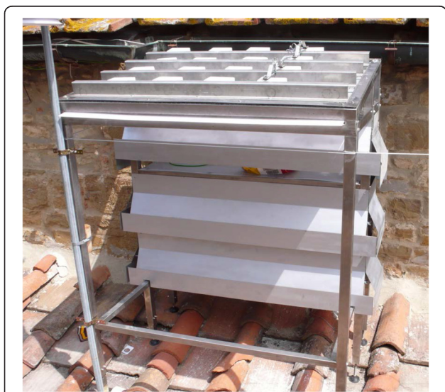
Figure 3 Galvanized rack used for the field exposure test (Santa Croce Basilica, Florence).
