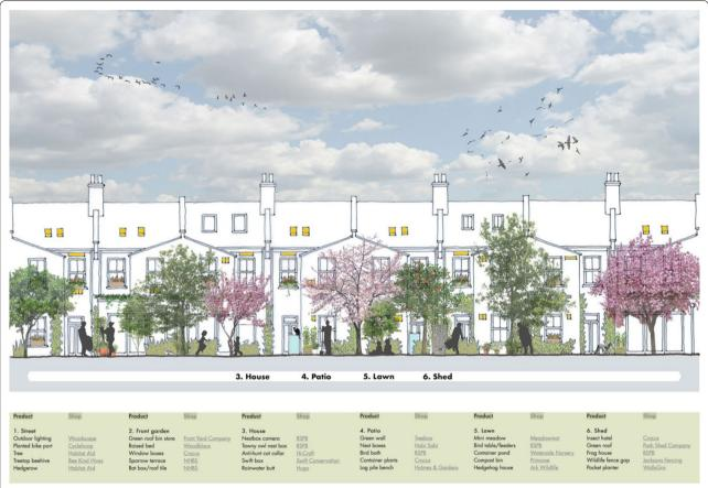
Fig. 4 Back garden elevation showing proposed typical street with adaptations for biodiversity, focusing on products (Siân & Jon Moxon & Viktoria Fenves)
