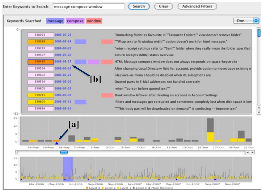
Fig. 10 Visualization of search results provided for searching “message compose window” in the software defect archive: (a) Most relevant defect indicated in the zoomed timeline; (b) Most relevant defect indicated in the information browser
