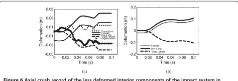
Figure 6 Axial crush record of the less deformed interior components of the impact system in normal mode (a) and reversed mode (b).
