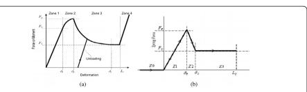
Figure 2 Illustration of; (a) the general component deformation pattern [7], and (b) the approximate force displacement diagram of the impact system.
