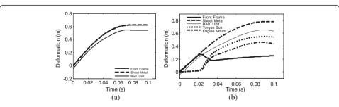
Figure 5 Axial crush record of the highly deformed front components of the impact system in normal mode (a) and reversed mode (b).
