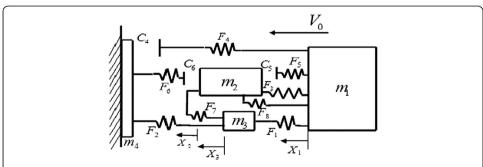
Figure 1 4-DOF LMS model in normal orientation for evaluation of the front structure in crash energy management.
