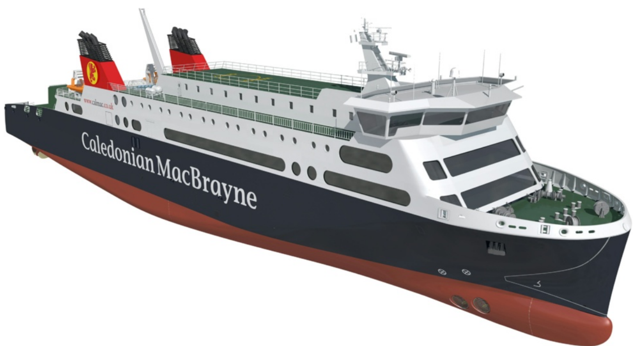
Figure 2 Design of the Caledonian MacBrayne. The figure shows one of the recent FSG RoPax ferry designs developed for the Scottish route between Ullapool and Stornoway. The bow door can be inferred by the white lines on the right hand side of the figure.
