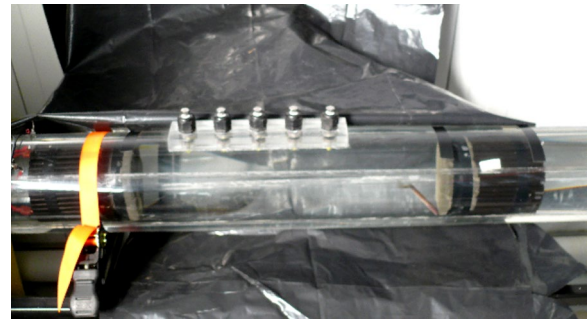
Fig. 2 Photograph of swim tube with larval lamprey at right (upstream) end
