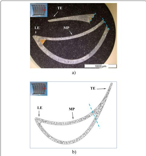
**Figure 3 Transversal section of a hollow vane. a)** Optical microscopy image of grain structure. **b)** Grain structure predicted by CAFE model. The dashed line on **b)** marks the cut plane on **a)**. TE stands for trailing edge, LE for leading edge and MP for middle part.
