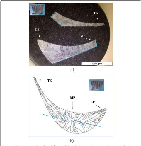
**Figure 5 Transversal section of a solid vane. a)** Optical microscopy image of grain structure. **b)** Grain structure predicted by CAFE model. The dashed lines on **b)** marks the cut planes on **a)**. TE stands for trailing edge, LE for leading edge and MP for middle part.
