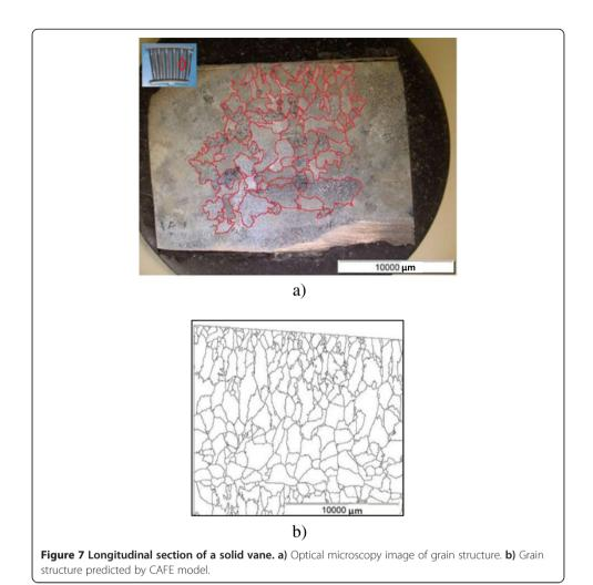
(Figure 7b) is similar to the experimental results. Microstructure with small grains close to the surface of solid vane (on the top of images), where solidification begins, is gradually transformed into microstructure with coarse grains when the mushy zone moves towards the central part of the solid vanes which is solidified in the last stage. It should be noted that the grain structure does not vary along the vane axis (horizontal axis in
