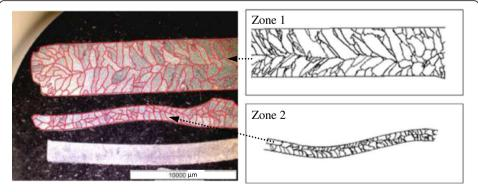
**Figure 9** Microstructure of longitudinal section in zones 1 and 2 of the bottom platform (Figure 8). Optical microscopy images (left) are compared with CAFE prediction (right).
