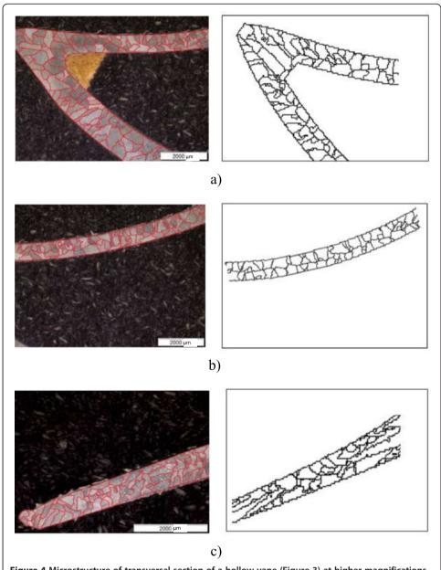
**Figure 4** Microstructure of transversal section of a hollow vane (Figure 3) at higher magnifications. Optical microscopy images (left) are compared with CAFE prediction (right): **a)** leading edge, **b)** middle part, and **c)** trailing edge.
