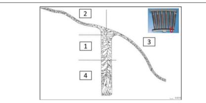
**Figure 8** Grain structure predicted by CAFE model on the longitudinal section of the bottom platform and four zones for microstructural analysis.
