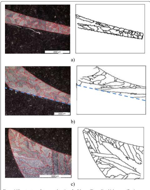
**Figure 6** Microstructure of transversal section of solid vane (Figure 5) at higher magnifications.
