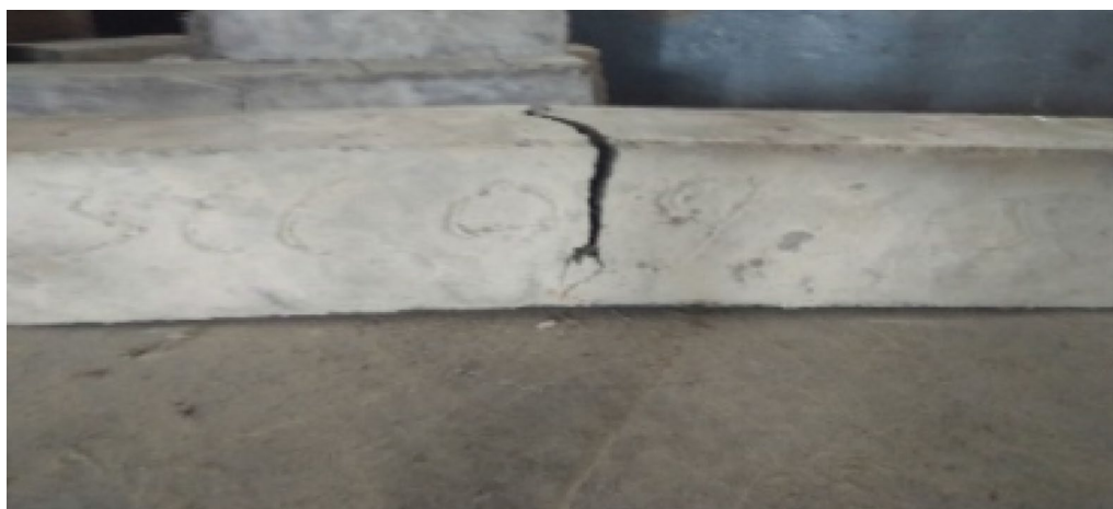
Fig. 11 Bridging effect of fiber (Sanjeev & Nitesh, 2020)
