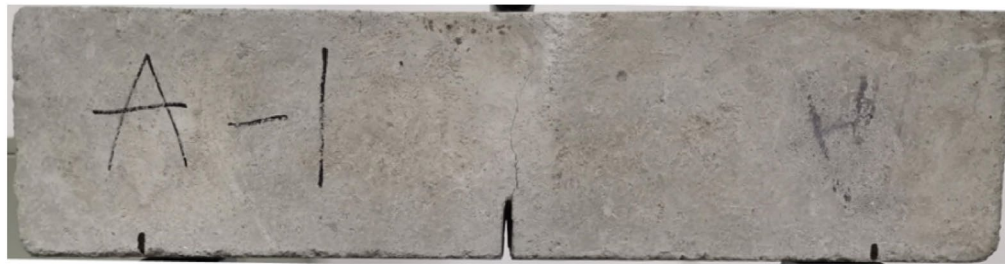
(a) Experimental crack propagation path
