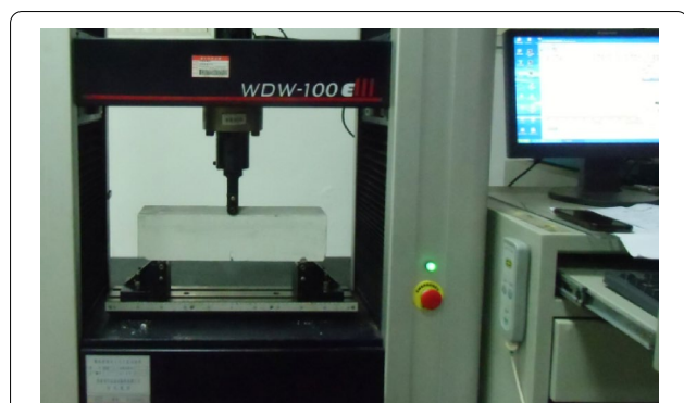
Fig. 4 Experimental setup of three-point bending
