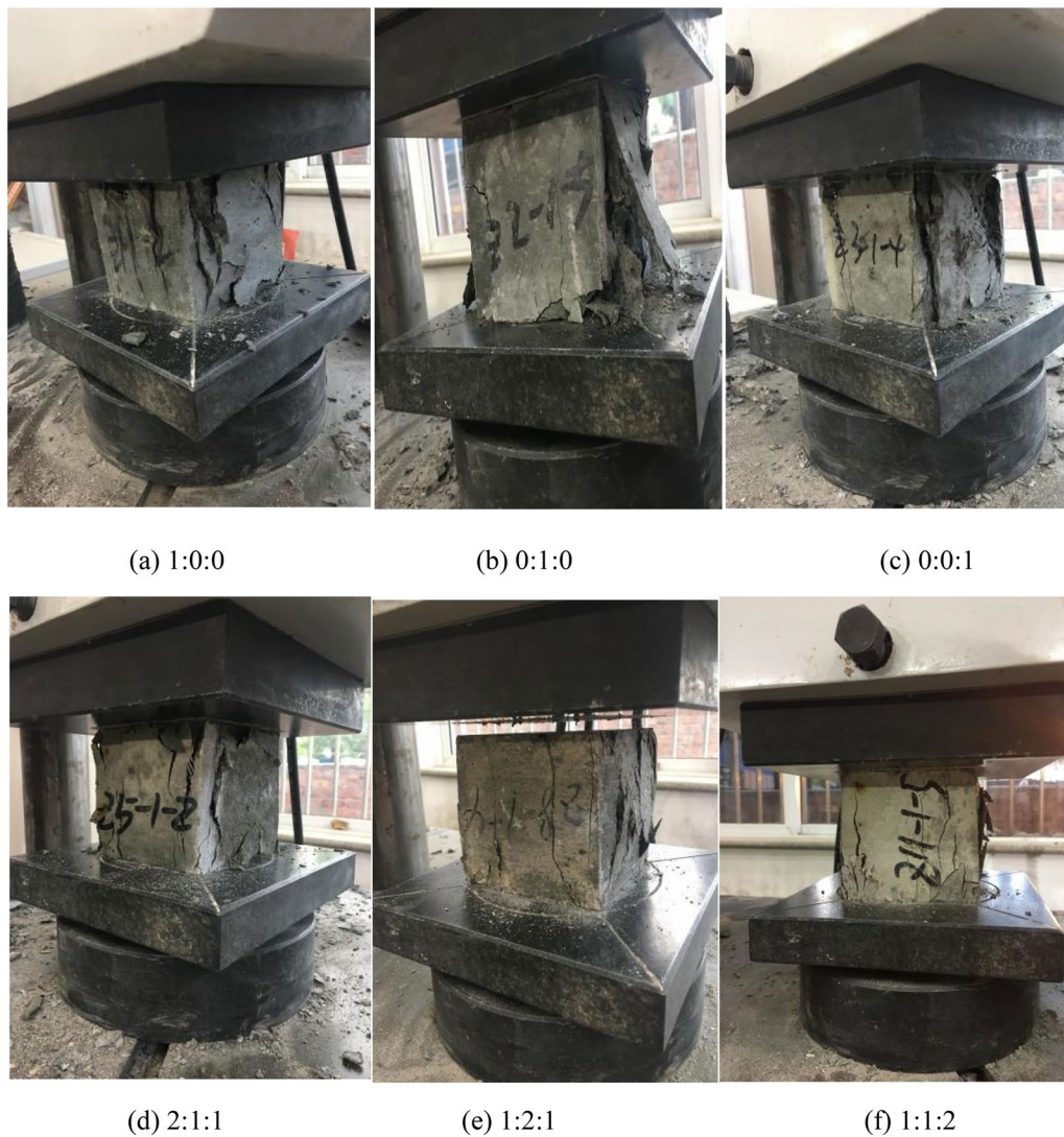
Fig.7 Failure modes based on the variation of additional ratio of fibers (CF: PPF: AF). a 1:0:0. b 0:1:0. c 0:0:1. d 2:1:1. e 1:2:1. f 1:1:2.
