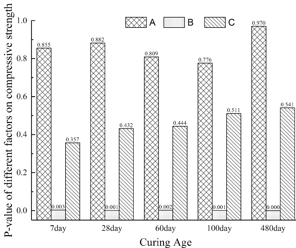
Fig. 15 P-value of different factors on compressive strength.
