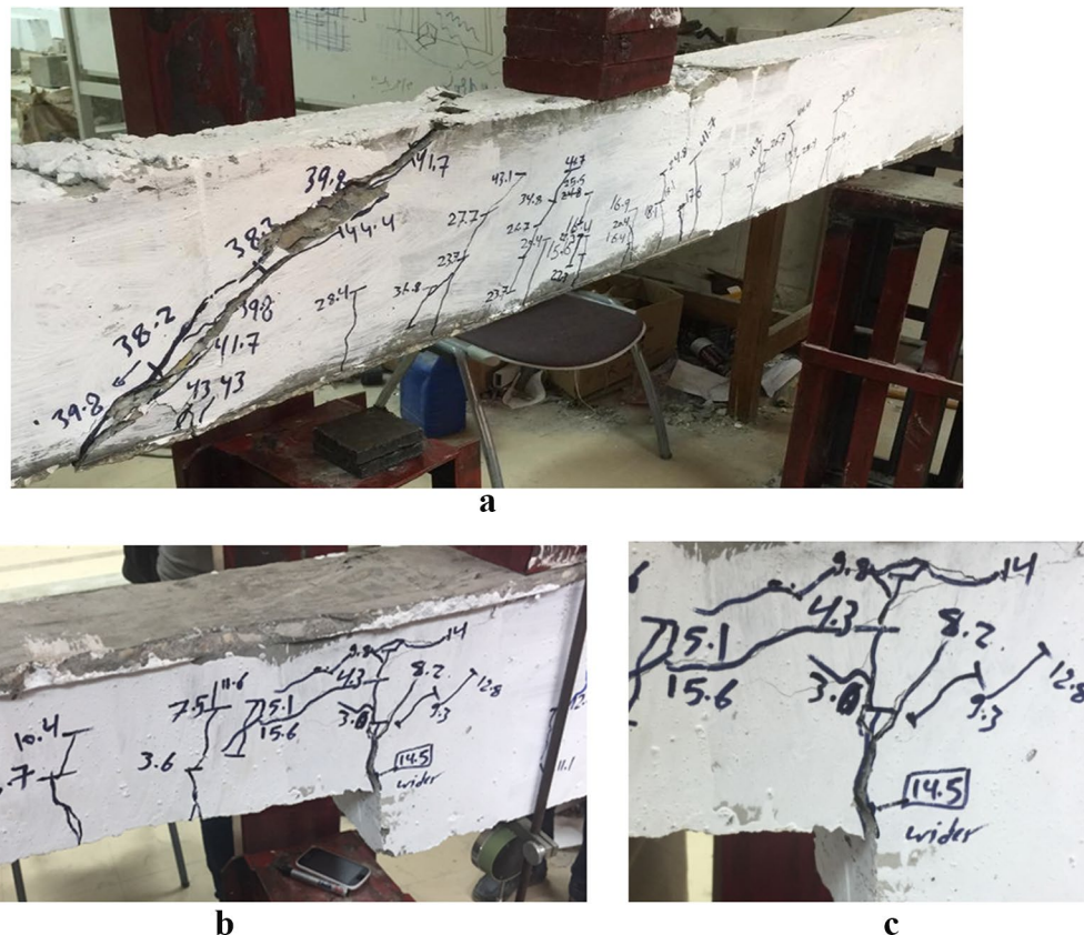
Fig. 5 Crack patterns of group G1: a side and top surfaces of Beam B0; b side, top surfaces of beam B2; c re-entrant corner of beam B2.
