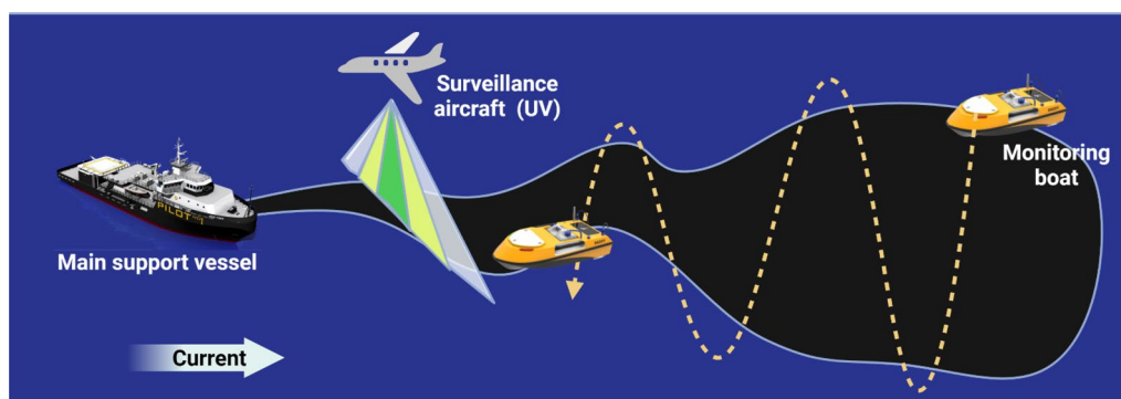
Fig. 8 A schematic diagram of the British test method. This method includes 1) the support vessel at anchor releasing and treating the oil in the tidal stream, 2) the sampling boat equipped with UV spectrofluorimetry, cruising through the oil trails and monitoring profiles of dispersed oil concentrations under the oil trail
