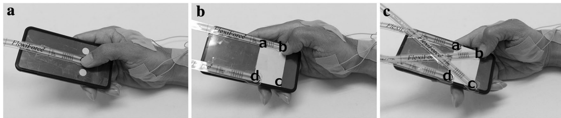
Fig. 2 Three tasks in the experiment. a Tapping task: large button task—button diameter of 9.0 mm, small button task—3.0 mm. b Moving task: ad-abduction task—orientation between a and c , flexion—extension task— b and d . c Circling task: clockwise task—direction a – b – c – d , counter-clockwise task: a – d – c – b
