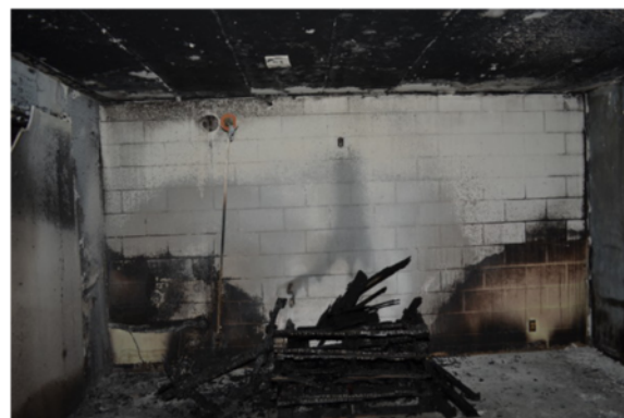
Fig. 6 Photograph of a Conical-Shaped Fire Pattern along a concrete block wall (fire origin was located under the stack of wooden pallets-fire test conducted at EKU by author)
