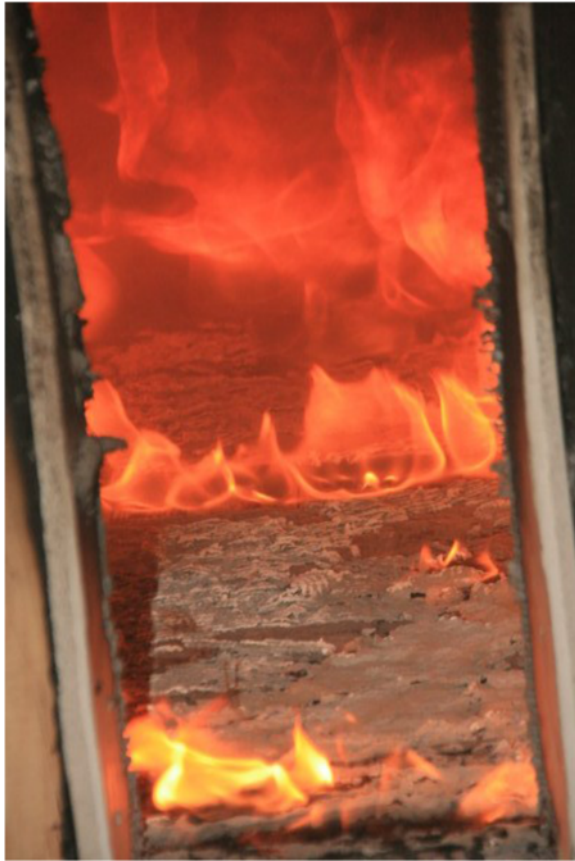
Fig. 8 Testing photograph for carpet pad seam generation of pattern similar to reported ignitable liquid pour showing burning in exposed surface resulting from carpet pad shrinkage (Wood et al. 2012)
