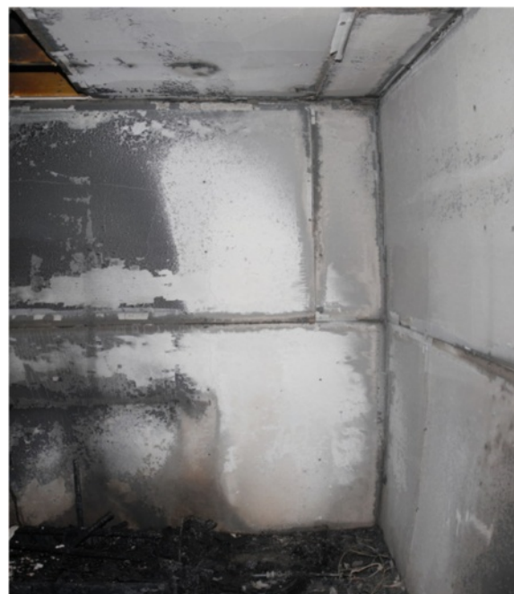
Fig. 11 Photograph of a Plume-Generated Fire Pattern (fire origin was located at the base of this damage-test conducted at ECU by author)
