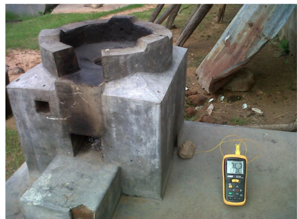
Fig. 9 Setup for temperature monitoring on the ash-removing hole of the Esperanza stove
