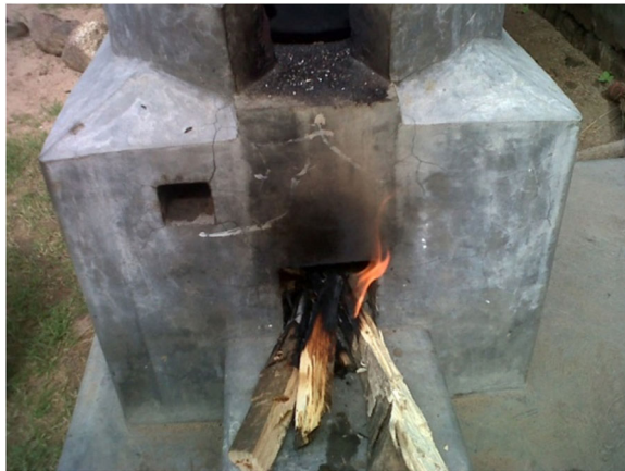
Fig. 6 The Esperanza stove in use with combustion outside the stove
