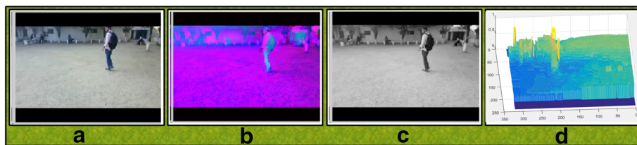
Fig. 3 Preprocessing results. a Original frame. b Contrast stretching. c Hue channel. d Mesh plot
