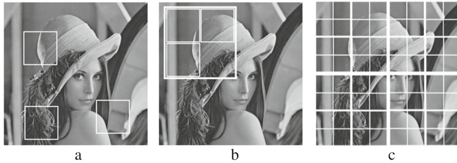
Fig. 8 Collecting a set of patches in PB-PCA filtering: a global PCA, b local PCA, and c hierarchical PCA
