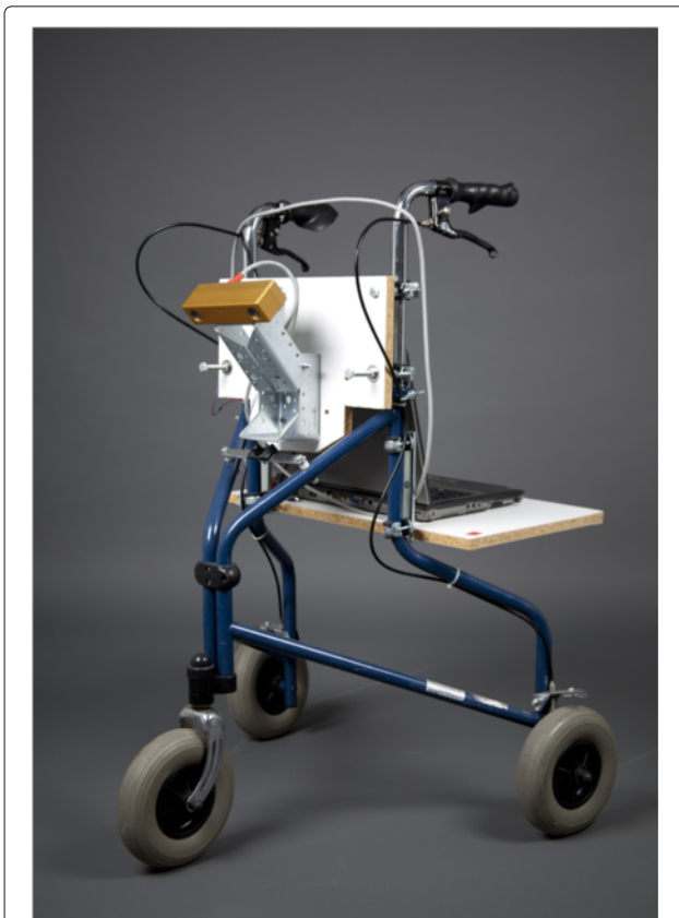
Fig. 5 Our experimental setup mounted with the Bumblebee2 stereo camera
