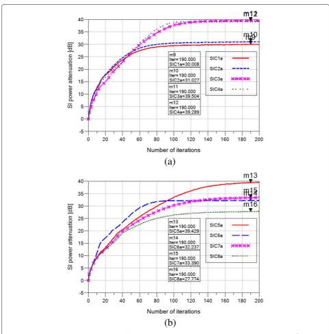
**Fig. 6** Additional SI cancelation provided by the RF canceler when the antenna isolation without reflections is 41 dB: **a** SI channel delay smaller or equal to RF canceler delay, **b** SI channel delay longer than RF canceler delay
