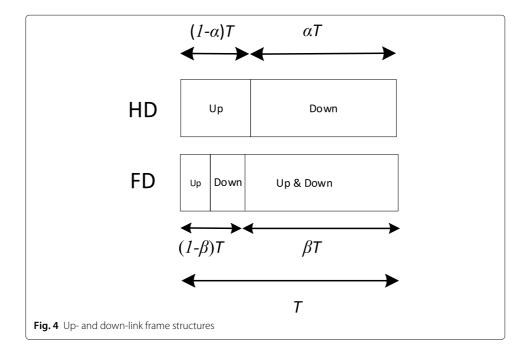
After the tuning has stopped and the SI channel has been estimated, the link is switched to the FD mode. Parameter  $\beta \in [0,1]$  defines the proportion of time spent in the HD and FD modes. If the HD mode requires the usage of additional FD specific pilots for SI channel estimation in digital baseband SI cancelation, the capacity is further reduced by the factor  $\kappa_{FD}$ . By taking into account of these factors, the sum rate of a FD link is
