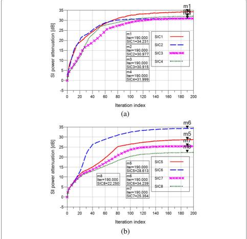
**Fig. 5** Additional SI cancelation provided by the RF canceler when the antenna isolation without reflections is 61 dB: **a** SI channel delay smaller or equal to RF canceler delay, **b** SI channel delay longer than RF canceler delay
