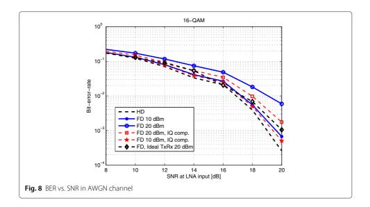
link. When the transmit power is increased to 20 dBm, the BER performance without IQ compensation is about 2 dB worse and with IQ compensation about 1 dB worse than the performance of an ideal FD receiver as is expected based on the results in Section 7.3.
